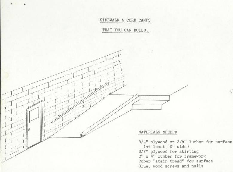
Wooden interior ramps need not be expensive. All they do require is sturdy construction, non-skid surface, correct slope, ample width, and a safety rail at the side(s). Most such ramps can be constructed for well under \$50.00 and are portable so they can be stored when not needed. The "when not needed" is a bit tricky because if you will watch, you'll see that most of the use is by able bodied people who find ramps easier to use than steps.
