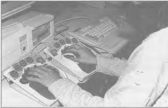
New solutions for persons with carpal tunnel syndrome include split keyboards (top) and "Data-hand."
